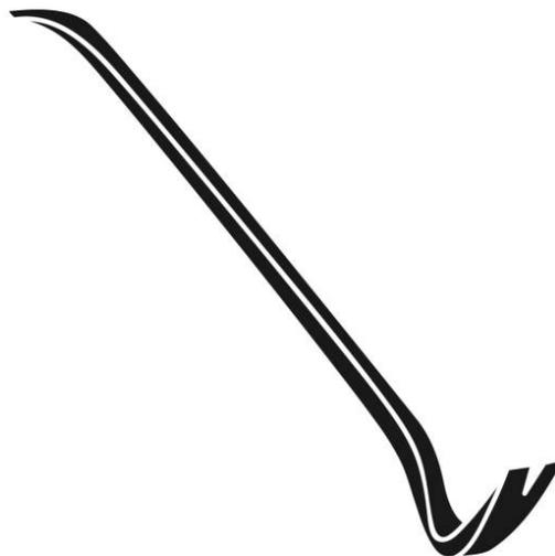
There are actually three main types of levers. The lever above is called a *class 1 lever*. In a class 1 lever, force is applied to the lever arm on one side of the fulcrum while on the other side of the fulcrum the load is moved.
